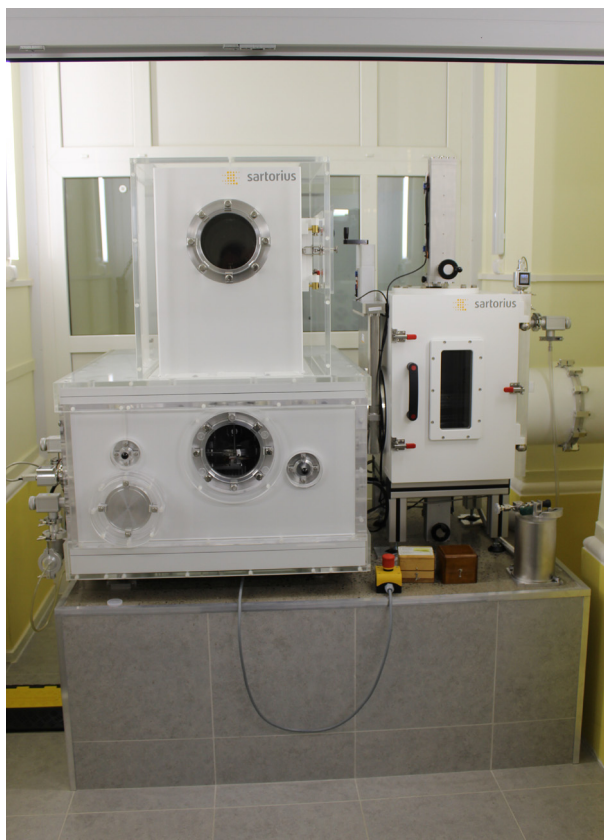
Fig. 1. The vacuum mass comparator Sartorius CCL 1007 (Germany) with VTS (vacuum transfer system)
