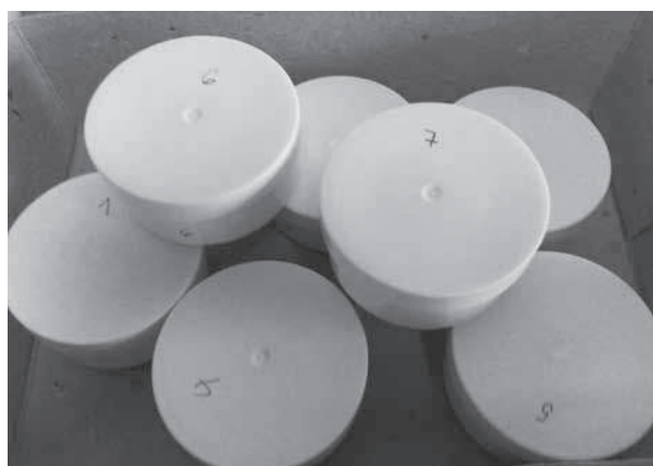
Figure 3. The reference material IONEX resin filled in seven identical containers
